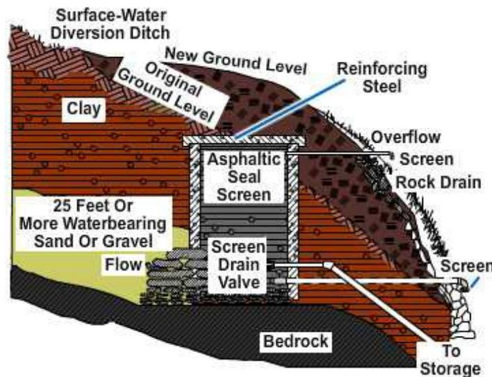
**Figure 5-9 — Protection of spring from surface contamination.**
