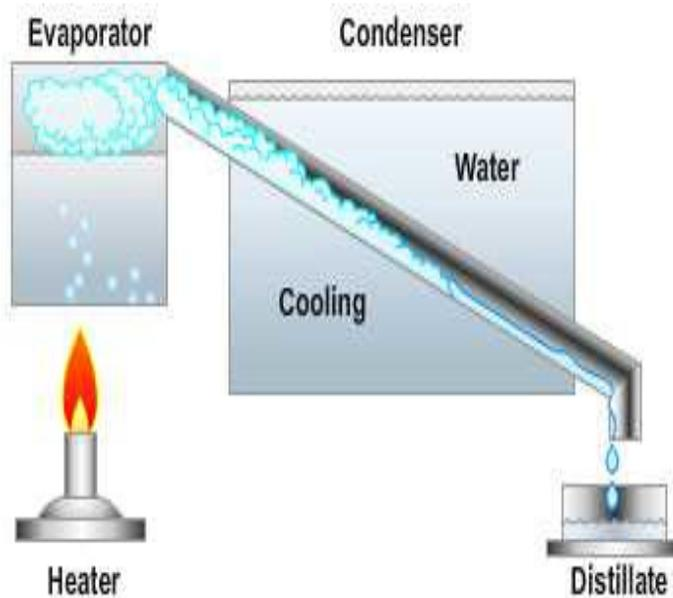
**Figure 5-10 — Distillation in its simplest form.**
