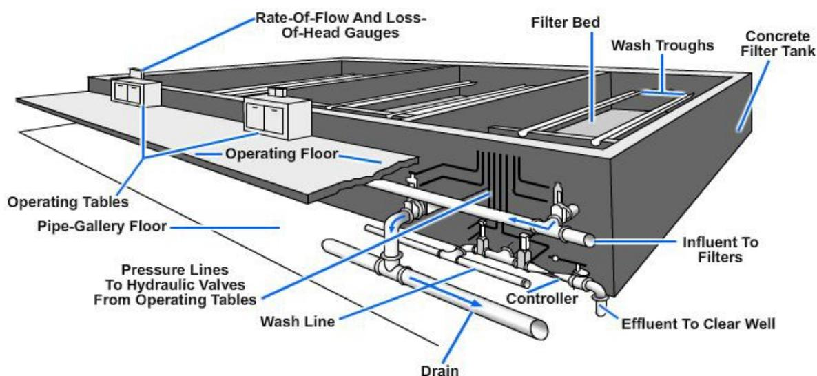
**Figure 9-15 — Types of gravity filters.**
