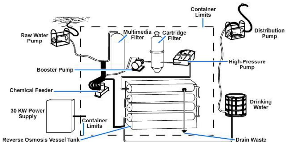
**Figure 5-13 — Water flow through the 600 gph ROWPU.**
