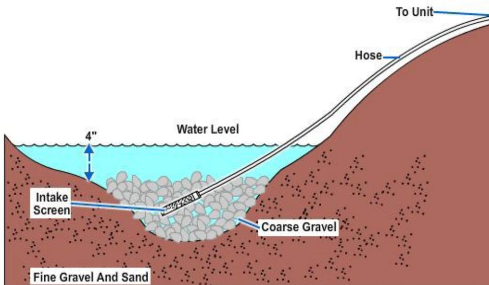
**Figure 5-6 — Methods for securing a surface intake.**
