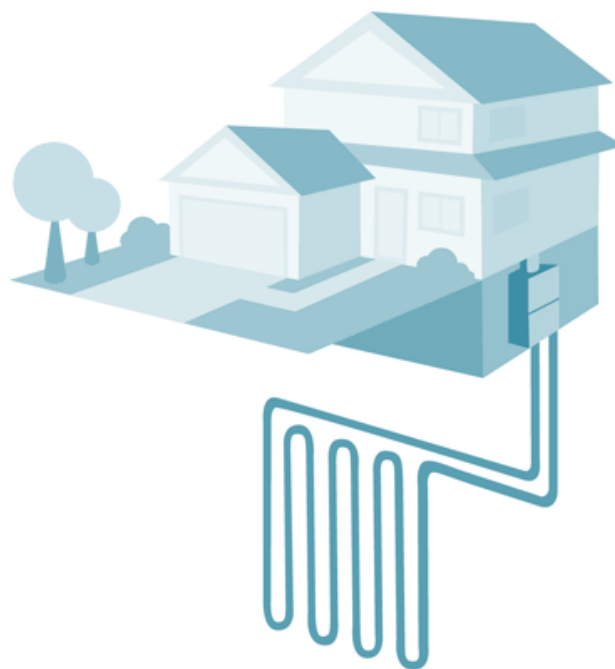
Figure 4. Vertical Ground Heat Exchanger
