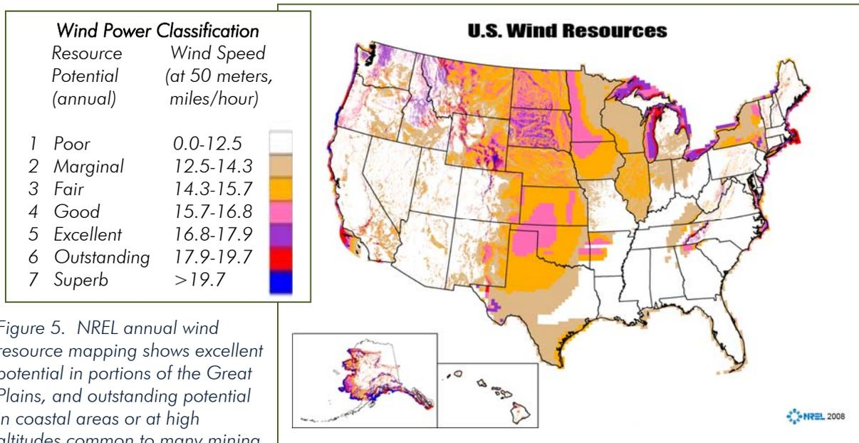
Figure 5. NREL annual wind resource mapping shows excellent potential in portions of the Great Plains, and outstanding potential in coastal areas or at high altitudes common to many mining sites requiring cleanup and reuse (U.S. DOE/NREL, 2008(b)).
