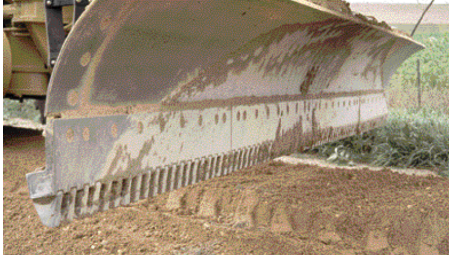
Examples of different types of replaceable bits for cutting edges.
