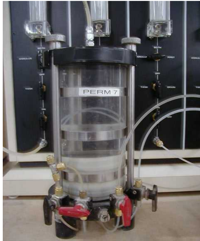
Figure 5-25. Flexible wall permeameter (Photograph courtesy of GeoComp Corporation).
