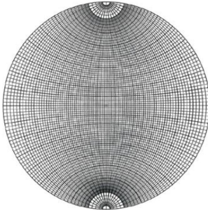
Figure C- 1. Wulff net, an equal-angle projection
