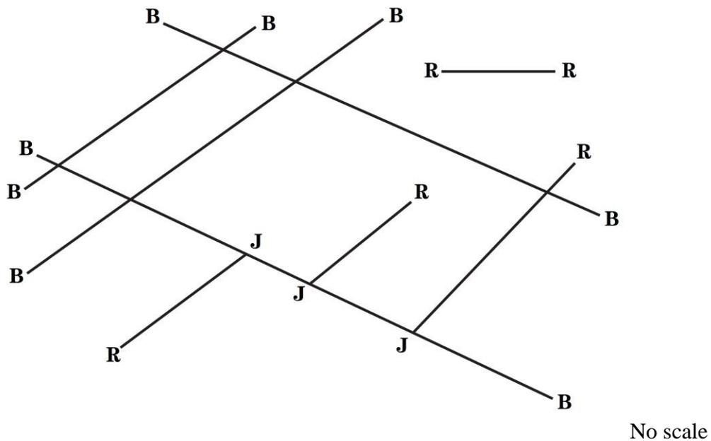
Figure 10. Types of joint ends in a rock outcrop
