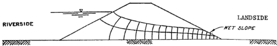
a. Homogeneous section on impervious foundation seepage emerging on landside slope
