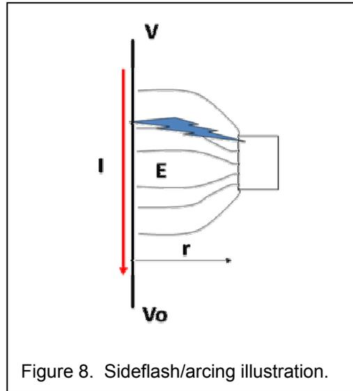
Figure 8. Sideflash/arcing illustration.
