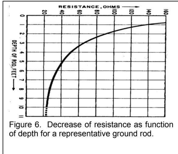
Figure 6. Decrease of resistance as function of depth for a representative ground rod.
