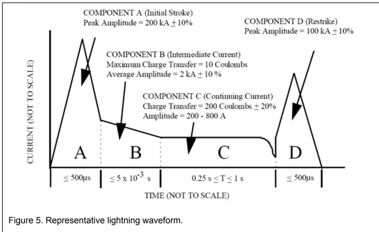
Figure 5. Representative lightning waveform.
