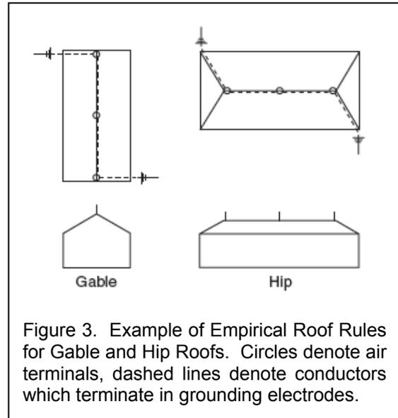
Figure 3. Example of Empirical Roof Rules for Gable and Hip Roofs. Circles denote air terminals, dashed lines denote conductors which terminate in grounding electrodes.
