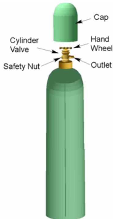
The oxygen volume in a cylinder is directly proportional to its pressure. In other words, if the original pressure of a full oxygen cylinder drops by 10% during welding, it means 1/10th of the cylinder contents have been consumed.
