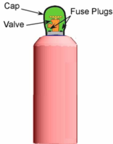
Acetylene is extremely **unstable** in its pure form at pressure above 15 PSI. This instability places special requirements on the storage of acetylene. Acetylene cylinders are packed with porous material (balsa wood, charcoal, corn pith, or portland cement) that is saturated with acetone to allow the safe storage of acetylene. These porous filler materials aid in the prevention of high-pressure gas pockets forming in the cylinder.
