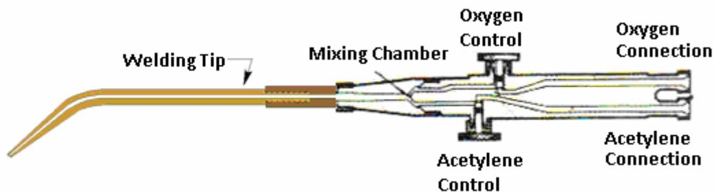
To change the power of the welding torch, it is only necessary to change the nozzle tip (size) and increase or decrease the gas pressures appropriately.
