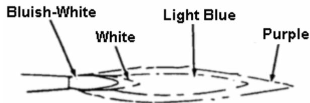
The feather is caused by incomplete combustion of the acetylene to cause an excess of carbon in the flame.
