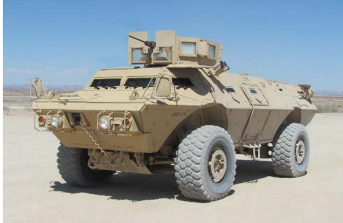
**Figure 1.** Mobile Strike Force Vehicle Armored Personnel Carrier
