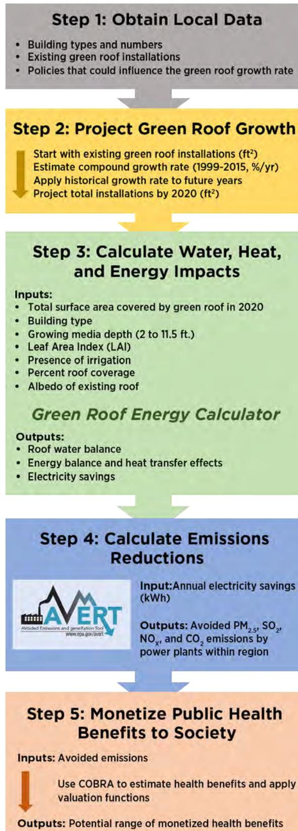
Figure 7. Analytical framework for estimating environmental effects of green roofs
