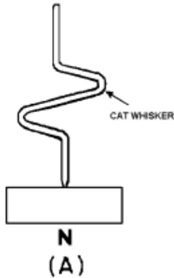
Figure 1-14A.—The point-contact type of diode construction.
