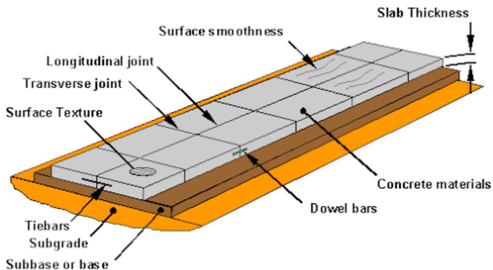
*Figure 18 Tie Bars and Dowel Bars in Rigid Pavements*
