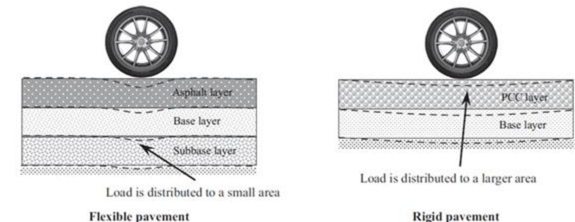
*Figure 3 Deformation Behaviour of Flexible and Rigid Pavements*
