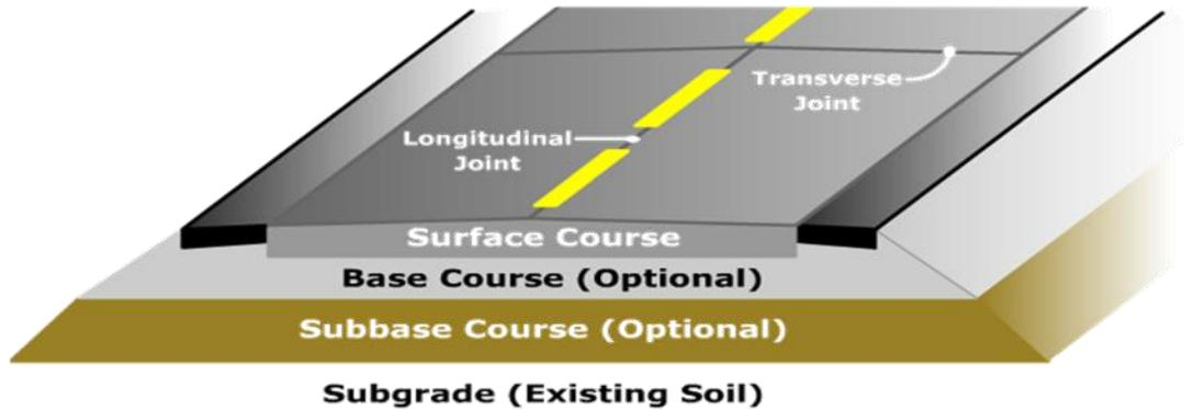
*Figure 11 Cross-Sectional View of Typical Rigid Pavements*
