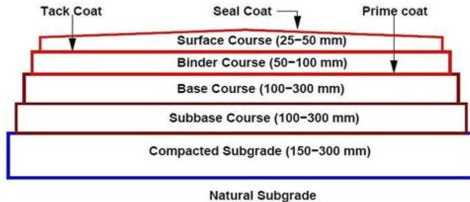
*Figure 64 Typical Layers of a Flexible Pavement*
