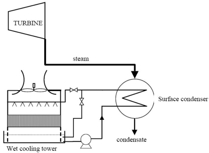
Figure 1 Schematic Diagram of Wet Heat Rejection System
