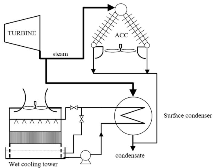
Figure 3 Schematic Diagram of Hybrid Heat Rejection System
