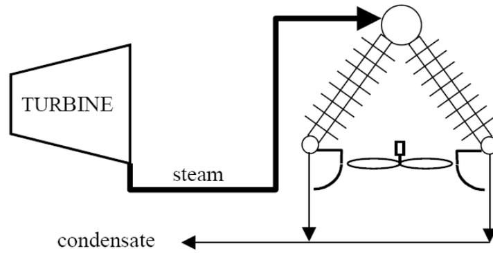
Figure 2 Schematic Diagram of Dry Heat Rejection System
