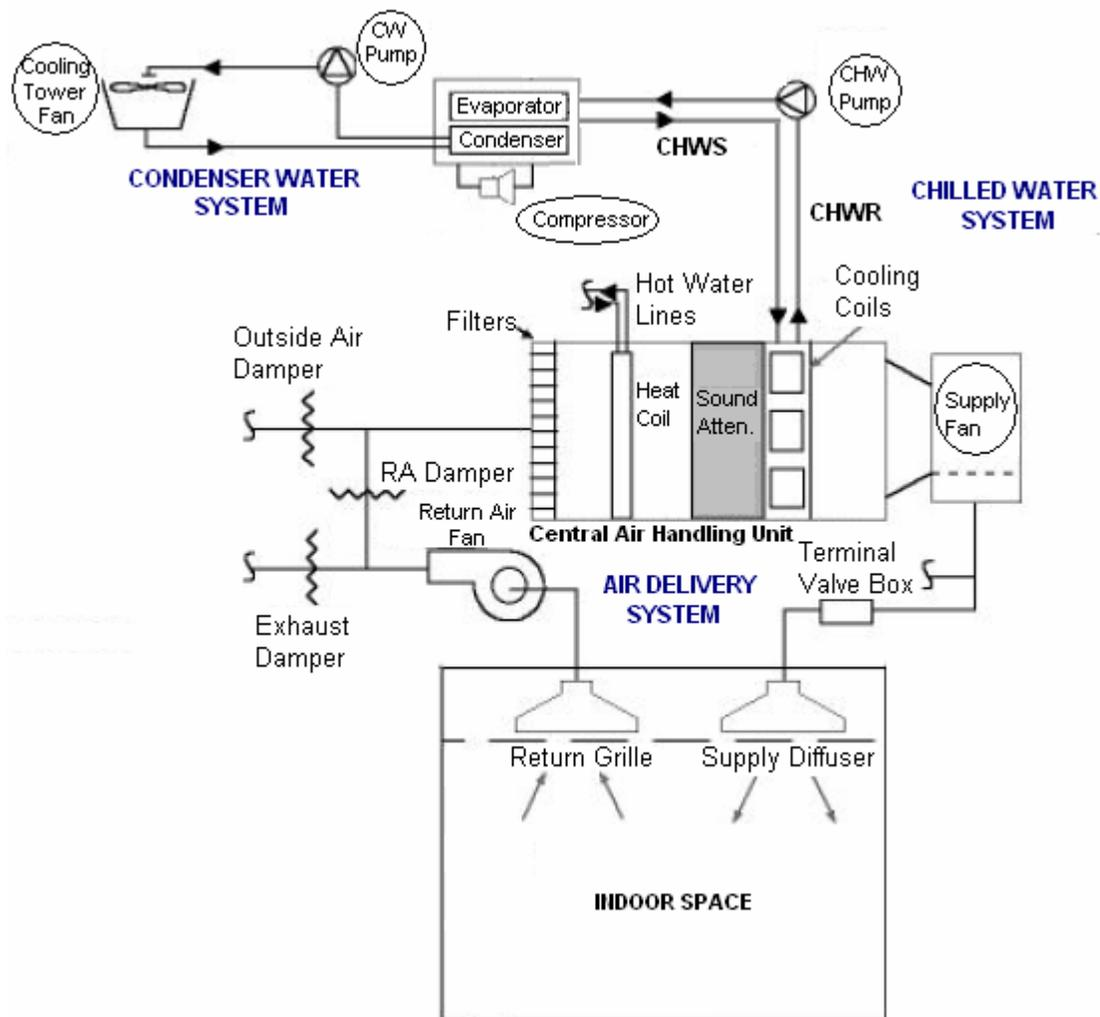
**Chilled Water System:** The chilled water system supplies chilled water for the cooling needs of all the building's air-handling units (AHUs). The system includes a chilled water pump which circulates the chilled water through the chiller's evaporator section and through the cooling coils of the AHUs. The system may have primary and secondary chilled water pumps in order to isolate the chiller(s) from the building: the primary pumps
