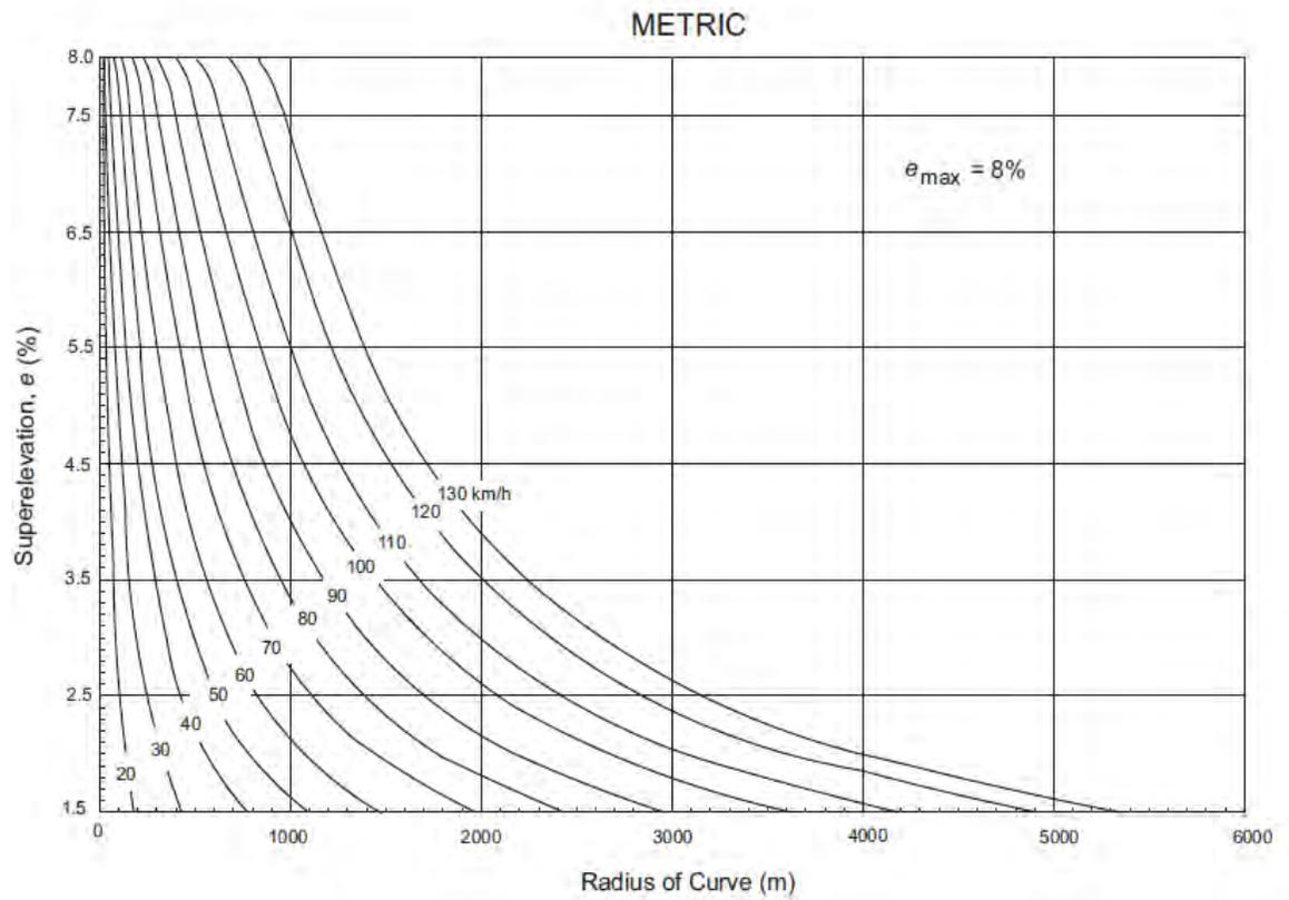
Figure 3.9 Design Superelevation Rates for  $e_{max}$  of 8% (SI)
