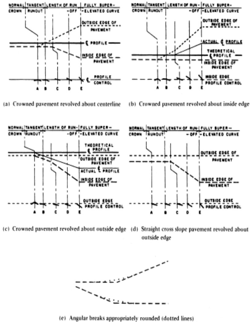
Figure 3.17 Diagrammatic Profiles Showing Methods of Attaining Superelevation for a Curve to the Right
