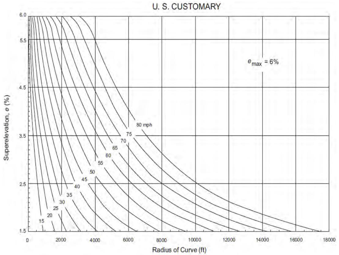
Figure 3.8 Design Superelevation Rates for  $e_{max}$  of 6% (US)
