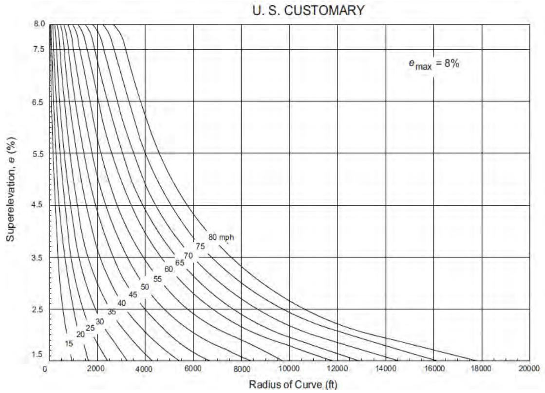
Figure 3.10 Design Superelevation Rates for  $e_{max}$  of 8% (US)
