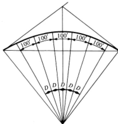
Figure 3.3 Arc Definition for a Circular Curve
