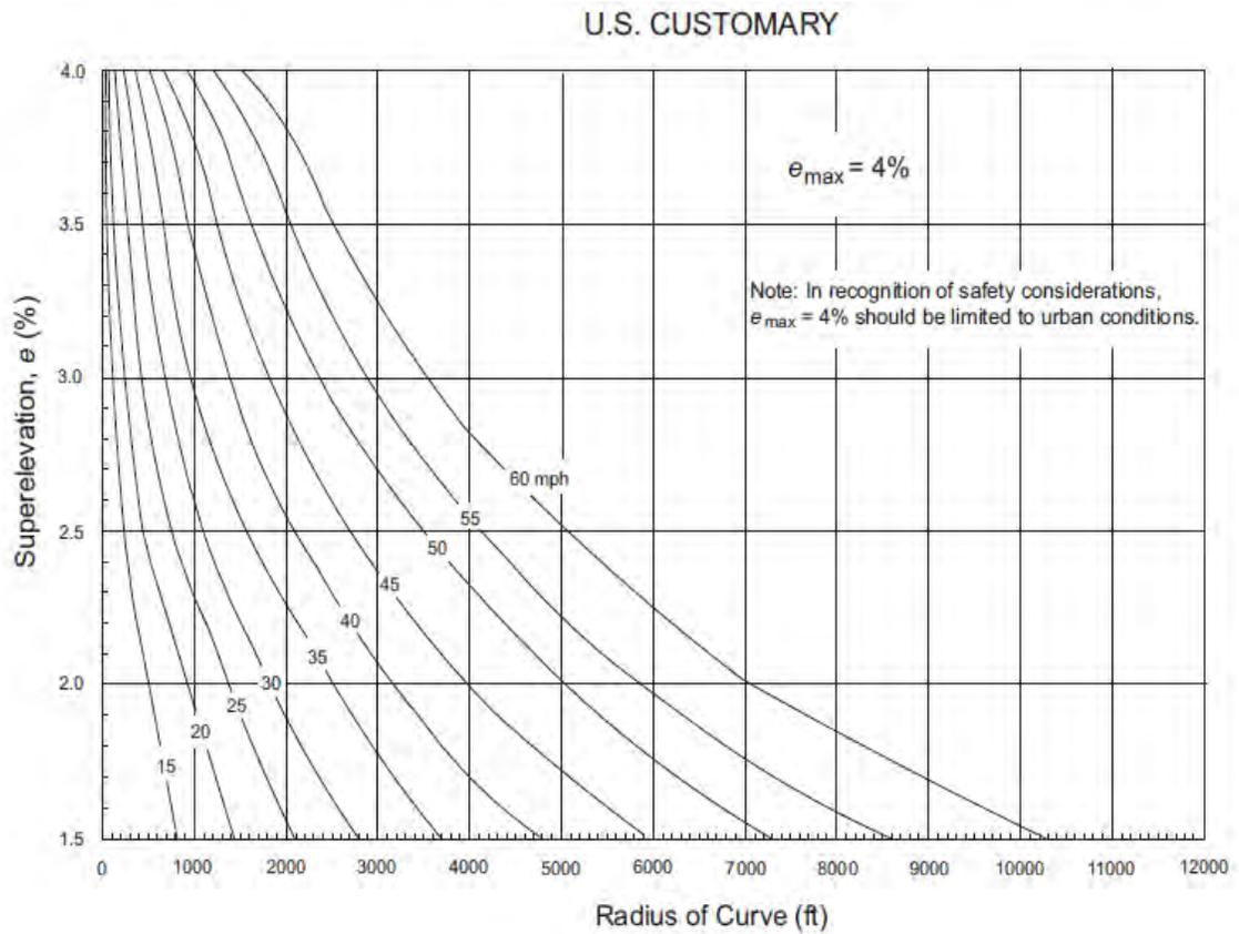
Figure 3.6 Design Superelevation Rates for  $e_{\max}$  of 4% (US)
