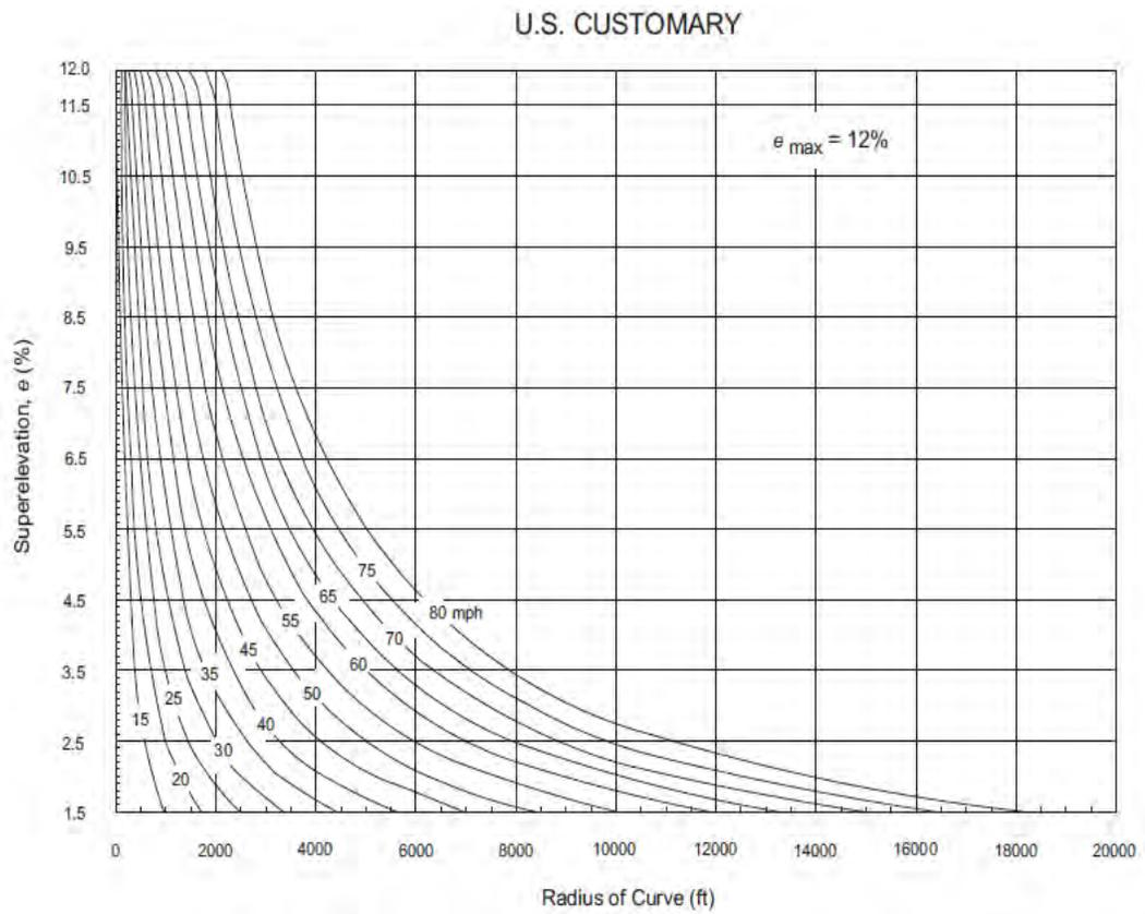
Figure 3.14 Design Superelevation Rates for  $e_{max}$  of 12% (US)
