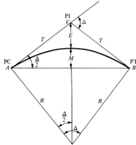
*R* = radius of circular curve      *PC* = point of curve
