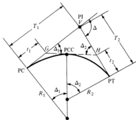
$R_1, R_2$  = radii of simple curves forming compound curve
