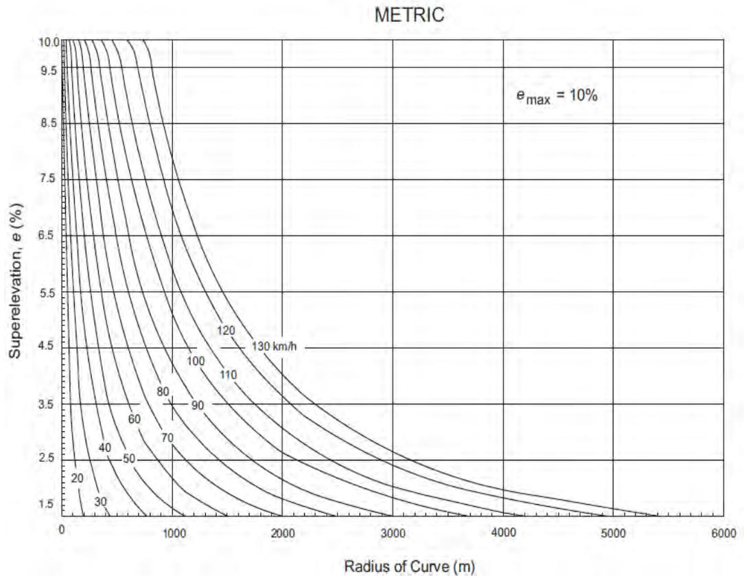
Figure 3.11 Design Superelevation Rates for  $e_{max}$  of 10% (SI)
