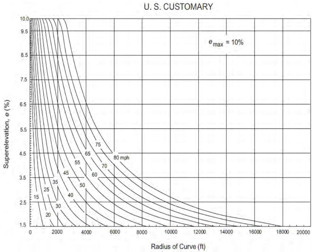
Figure 3.12 Design Superelevation Rates for  $e_{max}$  of 10% (US)
