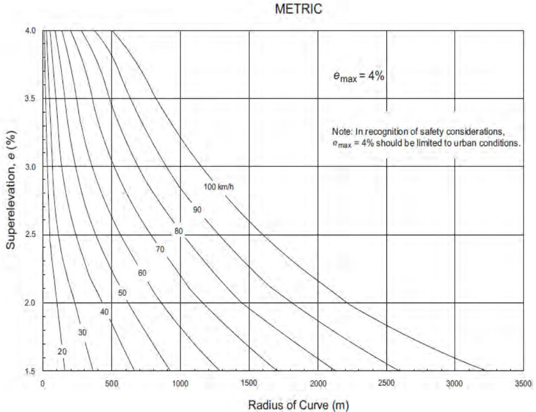
Figure 3.5 Design Superelevation Rates for  $e_{max}$  of 4% (SI)
