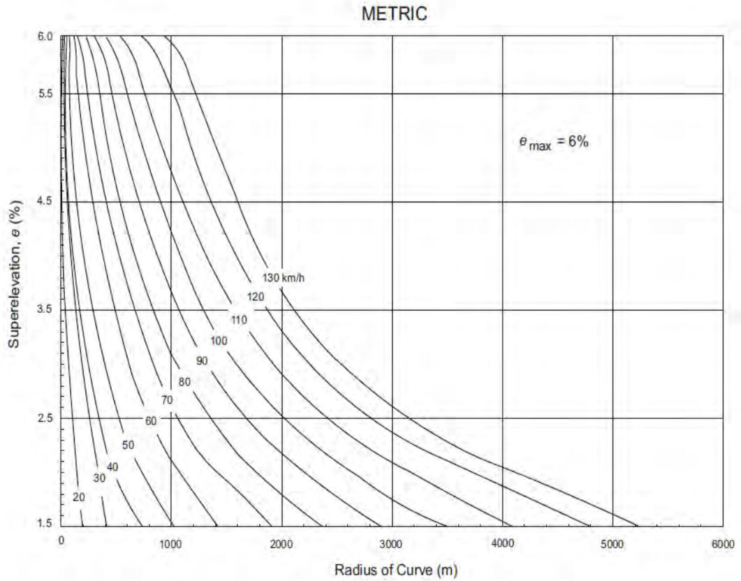
Figure 3.7 Design Superelevation Rates for  $e_{max}$  of 6% (SI)
