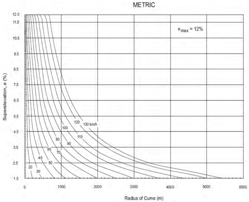
Figure 3.13 Design Superelevation Rates for  $e_{max}$  of 12% (SI)
