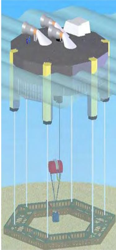
**Figure 3-4. The ORECon Multi Resonant Chambers (MRC) device deploys multiple OWCs around a 40-meter platform tethered to the sea floor offshore.**
