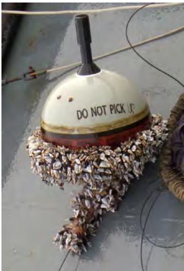
**Figure 3-14. Growth of biofouling organisms on a floating spherical buoy after 521 days at sea. Source: NOAA, [http://www.aoml.noaa.gov/phod/dac/gdp\\_drifter.html](http://www.aoml.noaa.gov/phod/dac/gdp_drifter.html)**
