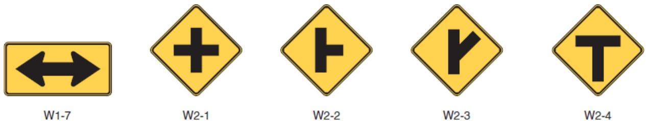
*Combination horizontal alignment/intersection signs* are used at intersections where side roads intersect a main road. These may be appropriate for locations where separate signs for intersections or curves might be misleading.
