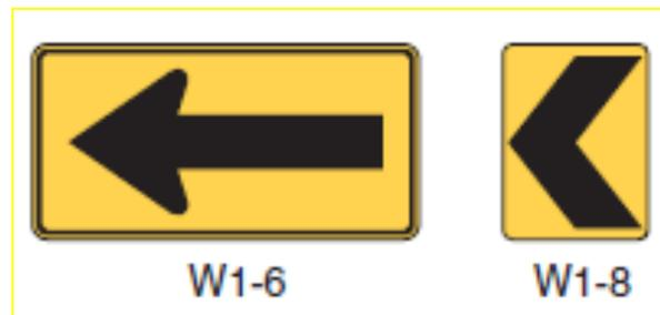
Chevrons need to be highly visible in order to provide adequate driver perception-reaction time. These signs should be installed on the outside of a turn or curve, in line with or at a right angle to approaching traffic. A minimum of two chevrons should always be visible by the road user. Three or more visible chevrons help drivers to visualize any changes in the alignment. Mounting chevrons on higher posts may be helpful for locations with limited sight distance or decreased visibility.
