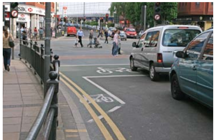
Figure 16. Railing is used to direct pedestrians to preferred crossing locations in London, United Kingdom.
