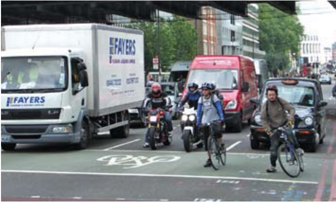
Figure 26. Bike boxes provide better visibility for turning bicyclists in London, United Kingdom.
