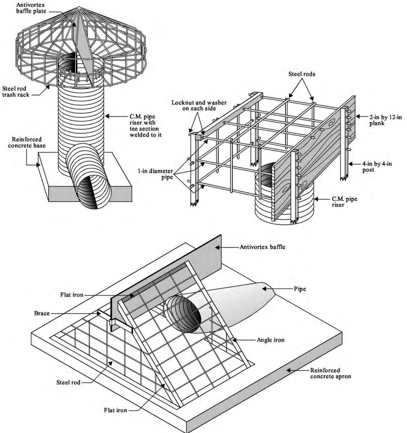
The required diameter for a hood-inlet pipe can be selected from table 14 or 15 after estimating the discharge capacity,  $Q$ , and determining the total head,  $H$ . The tables also show the minimum head,  $h$ , required above the invert or crest elevation of the pipe entrance. Unless you provide this minimum head, the pipe will not flow full.
