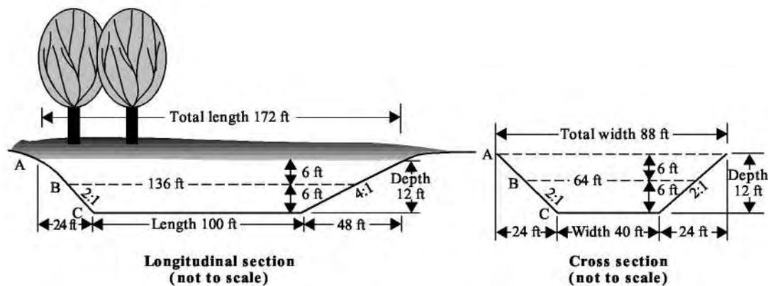
As an example, assume a pond with a depth,  $D$ , of 12 feet, a bottom width,  $W$ , of 40 feet, and a bottom length,  $L$ , of 100 feet as shown in figure 35. The side slope at the ramp end is 4:1, and the remaining slopes are 2:1. The volume of excavation,  $V$ , is computed as follows:
