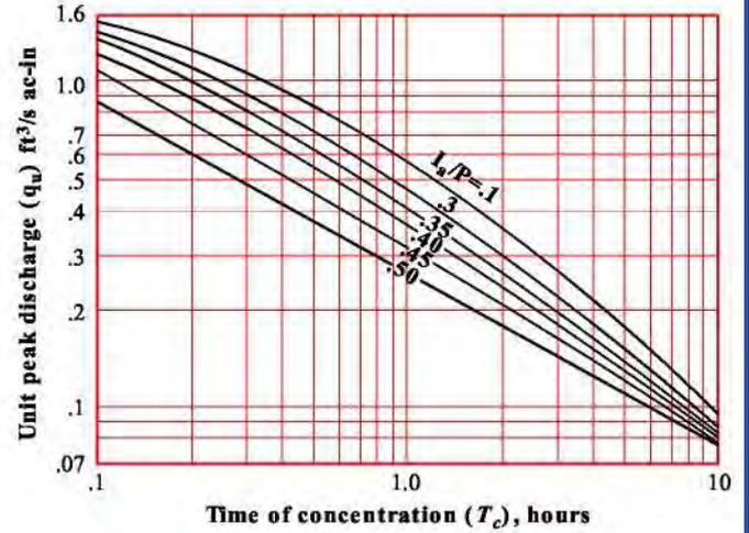
**Figure 17b** Unit peak discharge ( $q_u$ ) for Type IA storm distribution
