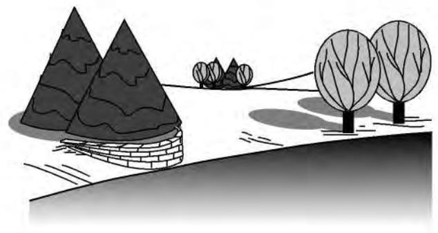
Removing all vegetation within the construction limits is not always necessary. Selected groupings of desirable plants can be kept. Trees and shrubs can often survive a 1- to 2-foot layer of graded fill over their root systems or they can be root-pruned in excavated areas. Tree wells and raised beds can also be used to retain vegetation (fig. 30).
