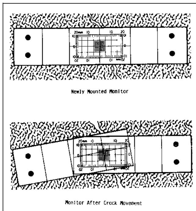
Figure 2-33. Crack monitor
