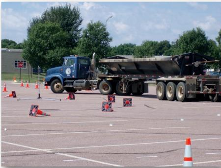
**Figure 3:** A wide-load tractor-trailer configuration vehicle navigating the mock driveable roundabout.
