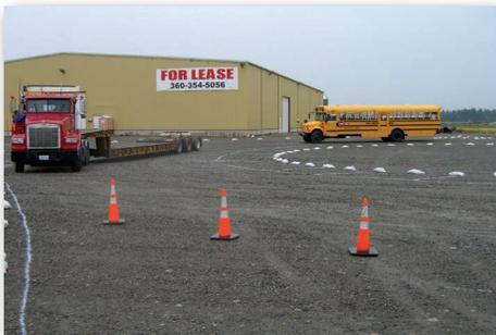
Figure 3: A large truck and a school bus navigating the mock roundabout.
