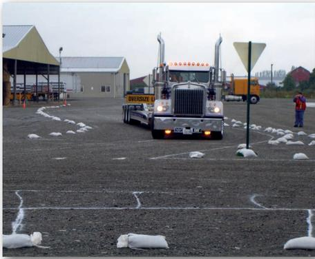
Figure 1: A large truck yielding before entering the mock roundabout.
