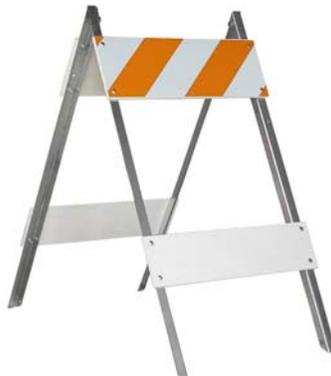
Type II Barricade has two horizontal retroreflective rails. The ballast shall not be placed on the top rails or any striped rails or higher than 13 inches above the driving surface. The barricade shall be 36” in height and 24” in width. The rails shall be 8” in height.
