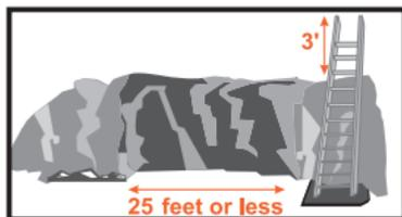
A competent person must inspect trenches daily and when conditions change. An unprotected trench is an early grave. Do not enter an unprotected trench.
