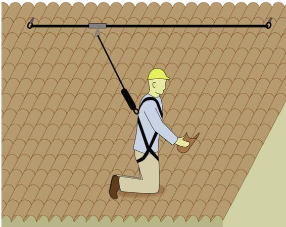
**Leave anchors in place:** Where practical, consider leaving roof anchors in place. It will make the current job simpler and reduce the burden for roofers in the future.
