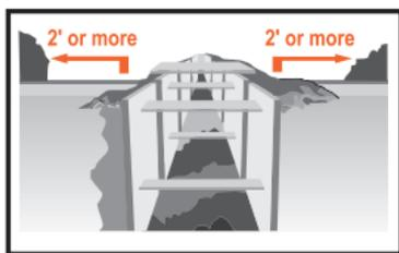
A safe way to exit must be provided within 25 feet of workers in a trench.
