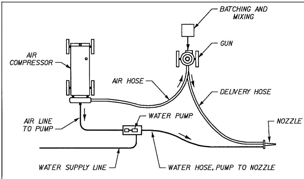
Figure 4-3. Typical plant layout for dry-mix shotcreting (Crom 1966; copyright permission granted by ACI)
