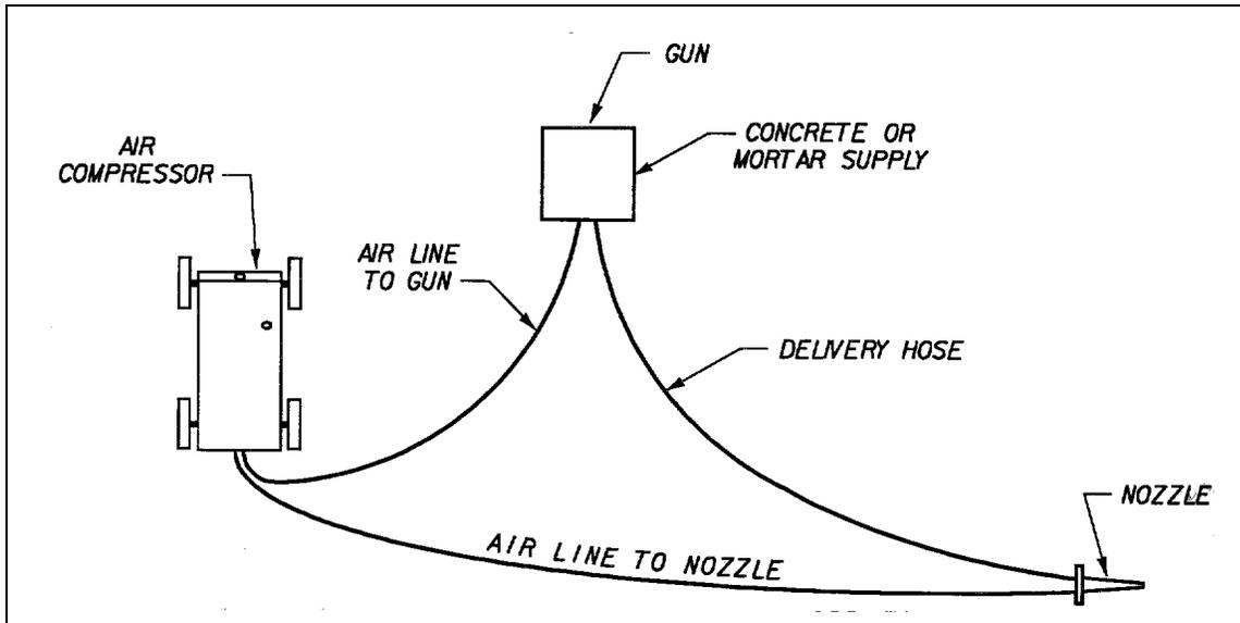
Figure 4-6. Typical plant layout for wet-mix pneumatic-feed equipment
