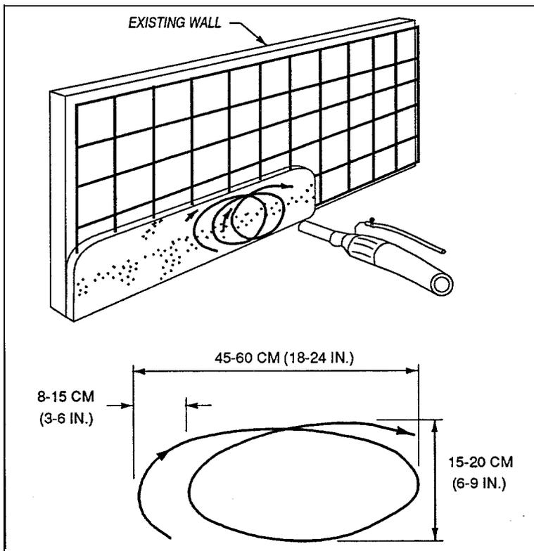
Figure 6-2. Shotcrete nozzle motion (after Ryan 1973)
