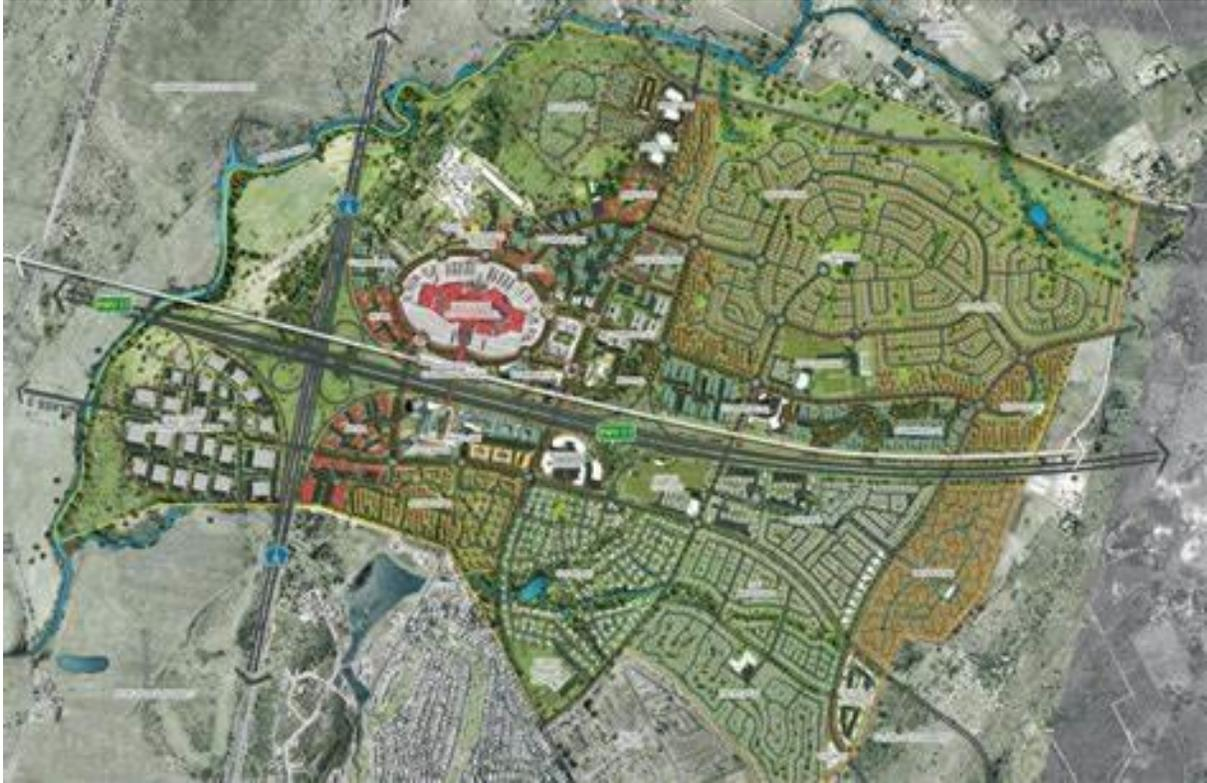
The following illustration shows how arterial roadways are used to “feed” the collector roads serving the local roads. The local roads then “feed” the neighborhood cul-de-sacs. A transit road is also built into the roadway system.
