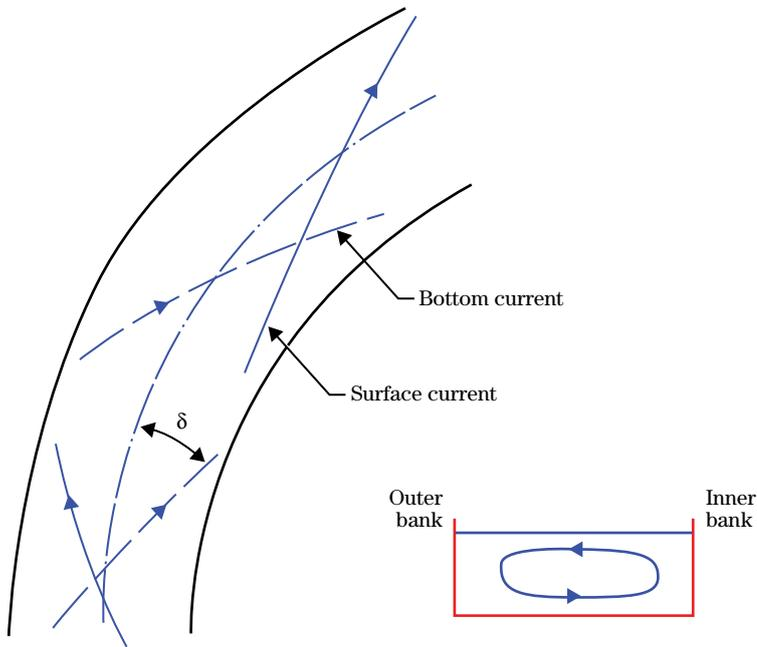
**Figure 6-13** Flow characteristics for a typical reach
