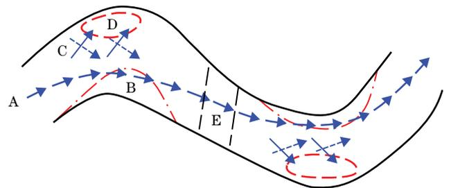
currents angle into the bank and undercurrents move away from the bank, a zone of downwelling results at point D. The low bed load gives the stream a scouring tendency. Toward the inflection point of the meander, flow with a low bed-load supply enters a contracted reach at E that is steeper and shallower, and regains its scouring capacity. Riffles form and, as the highest velocity vectors cut from one point bar toe to the toe of the next downstream bar, riffles are often skewed to the banks.
