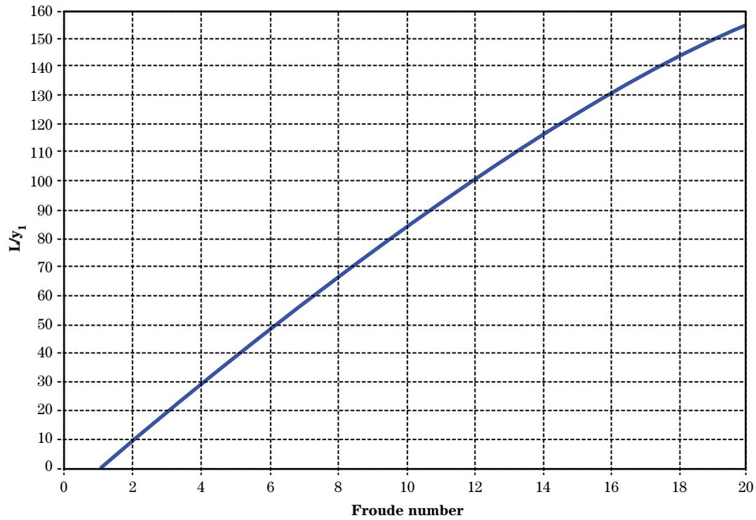
**Figure 6-21** Parameters involved with modeling a hydraulic jump
