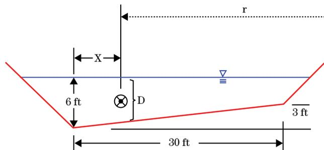
To find X, the flow area left of the centroid must be equated to that on the right:
