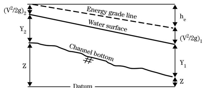
The energy loss includes friction losses (usually evaluated with Manning's equation) and losses associated with changes in cross-sectional areas and velocities. This is represented in equation 6-56:
