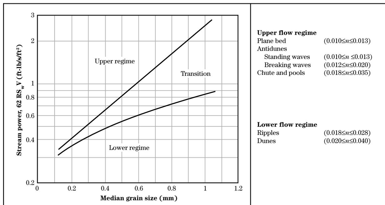
Figure 6–10 (Arcement and Schneider 1990) indicates the general bedforms for increasing stream power.
