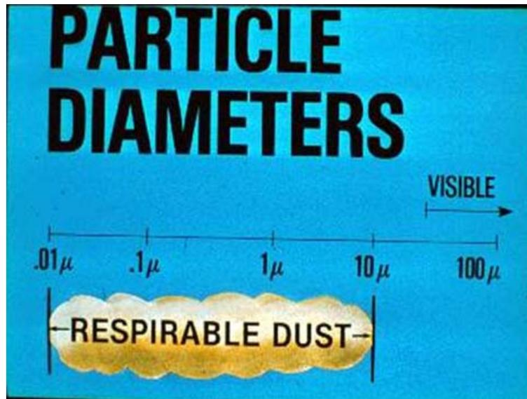
**Figure 19.** Range of size of dust particles
