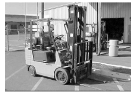
Safety features include an overhead guard.
