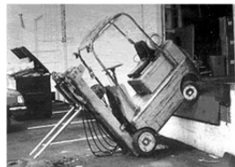
Forklift driven off loading dock.
