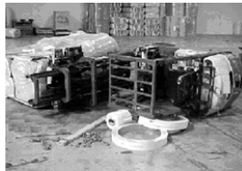
Overturned forklift resulted in fatality.
