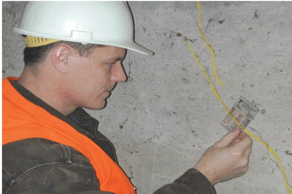
**Figure 2.2.10** Crack Comparator Card
