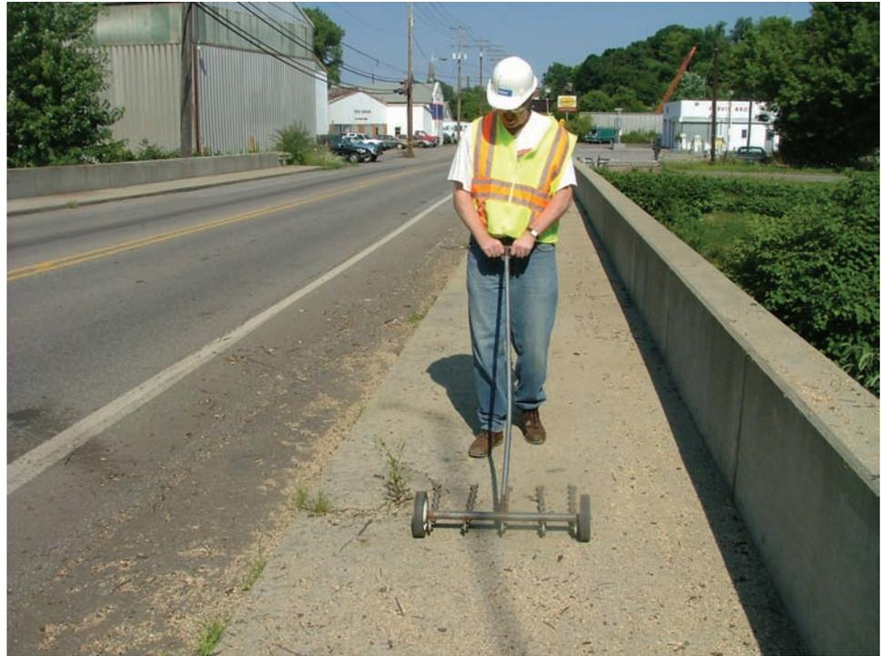
**Figure 2.2.29:** Inspector Using a Chain Drag
