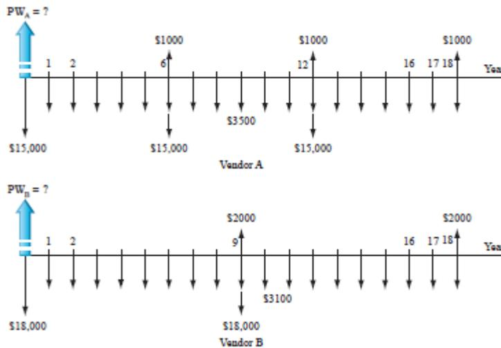
**Figure 25 Cash Flow Diagram for Different-Life Alternatives, Example 24**
