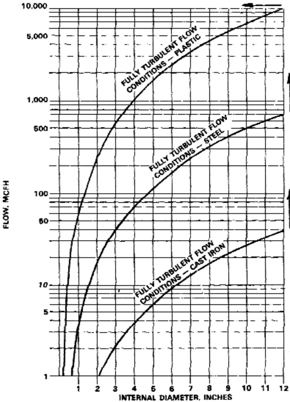
BASED UPON: IGT DISTRIBUTION EQUATION AND FULLY TURBULENT EQUATION,
