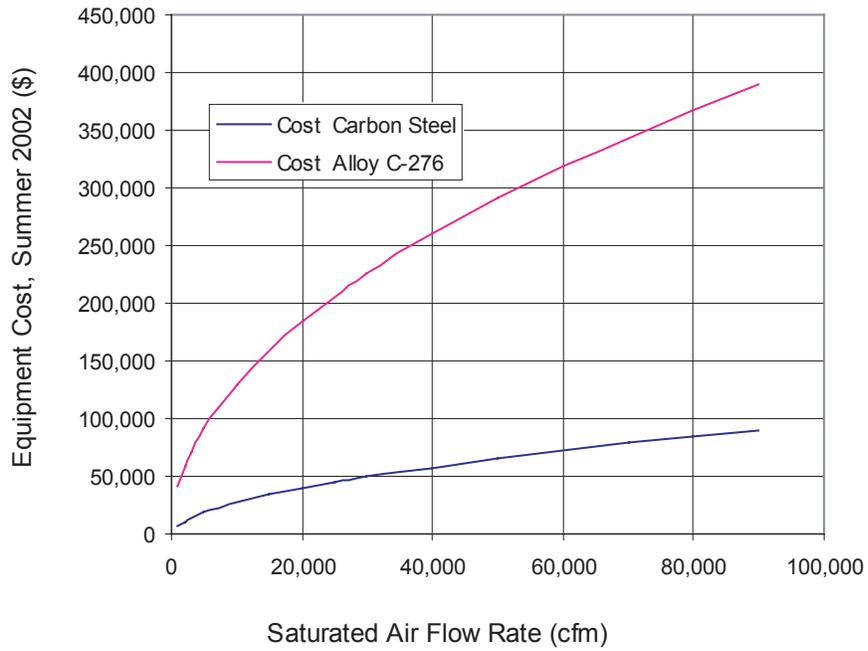
**Figure 2.16:** Equipment Costs for High Energy Venturi
