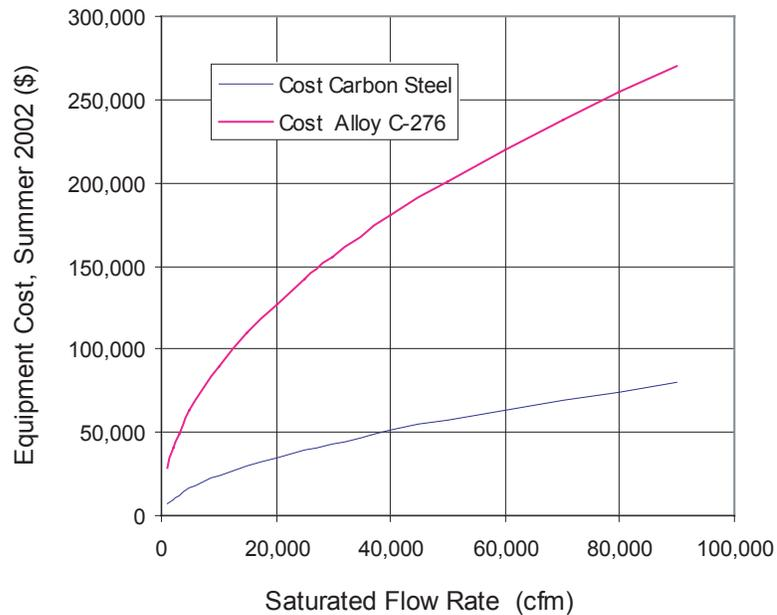
**Figure 2.15:** Equipment Costs for Low Energy Venturi
