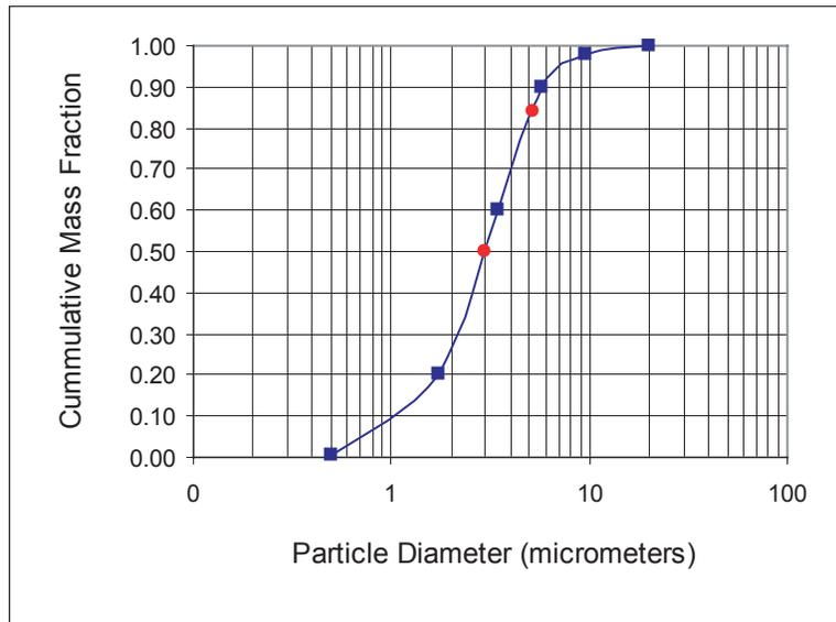
**Figure 2.18:** Particle Size Distribution for Sludge Incinerator
