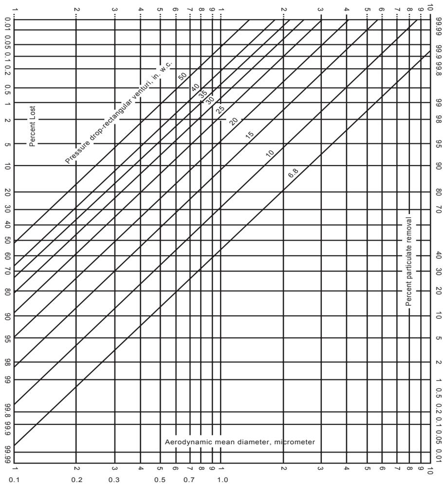
**Figure 2.6:** Approximate Collection Efficiencies of Particles in the 0.1-10  $\mu\text{m}$  Diameter Range at Venturi Pressure Drops in the 6.8-50 in.  $\text{H}_2\text{O}$  Range [2]
