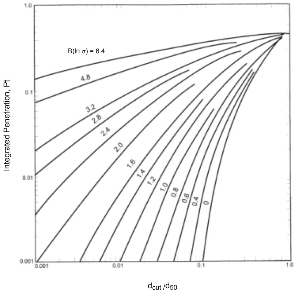
**Figure 2.12:** Cut Diameter as a Function of Cut Ratio and Standard Deviation of the Particle Size Distribution [20]
