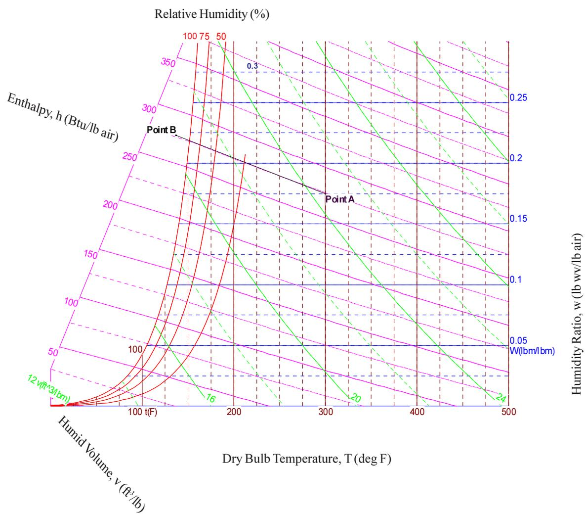
**Figure 2.9:** Psychrometric Chart at Standard Pressure, 14.7 psi
