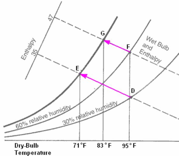
*Evaporative cooling process with hot dry air from points D to E and with hot humid air from points F to G. Notice greater evaporative cooling capacity with dry air.*
