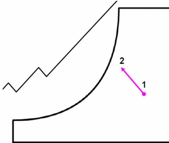
The evaporative cooling process is commonly employed to reduce the dry bulb temperature of the air without refrigeration. It is a constant wet bulb process of reducing dry bulb temperature. The hardware used to achieve this process usually consists of the basic components of the adiabatic saturation chamber plus some type of device to amplify the interface surface area between the water reservoir and the air, such as wetted wick, matting, plates, spray, etc.
