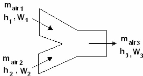
In most cases, heat loss from the system is negligible and the system can be modeled as adiabatic. On a psychrometric chart, the condition of the exiting air stream must be on the line connecting the incoming air streams. The distance along that line is determined by the ratio of the mass flow rates of the incoming streams.
