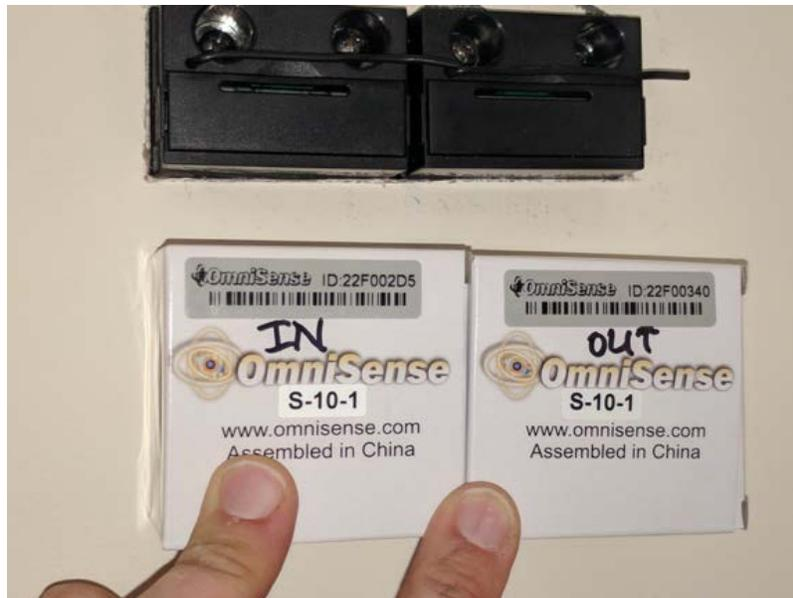
Figure 13. Typical moisture sensor placement in SPS wall showing interior surface and exterior surface panel depths
