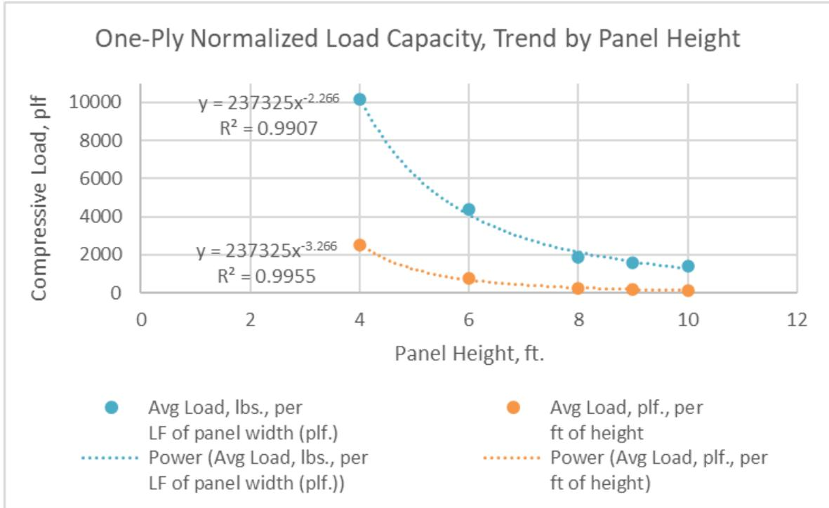
Figure 24. 1-ply load capacity trend by panel height
