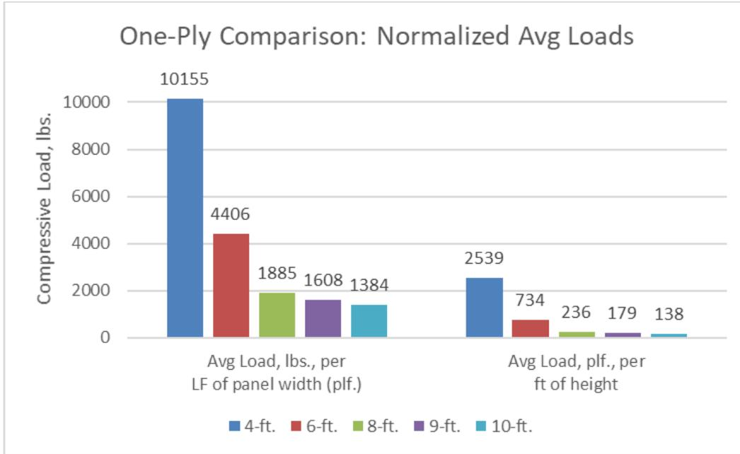
**Figure 17. Normalized average loads for 1-ply—all specimen heights**
