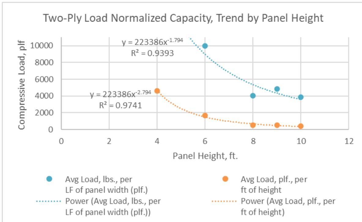
Figure 25. 2-ply load capacity trend by panel height
