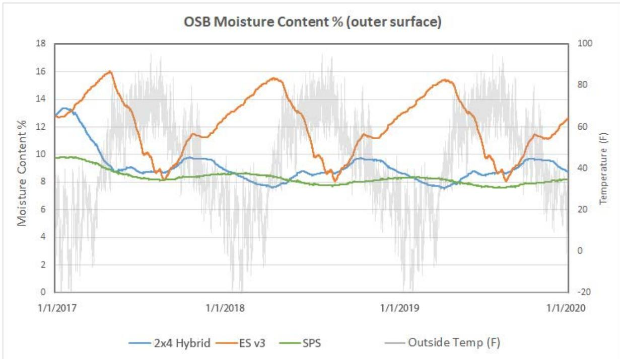
Figure 22. WUFI Plus simulation, OSB inner and outer surface moisture contents over 3 years
