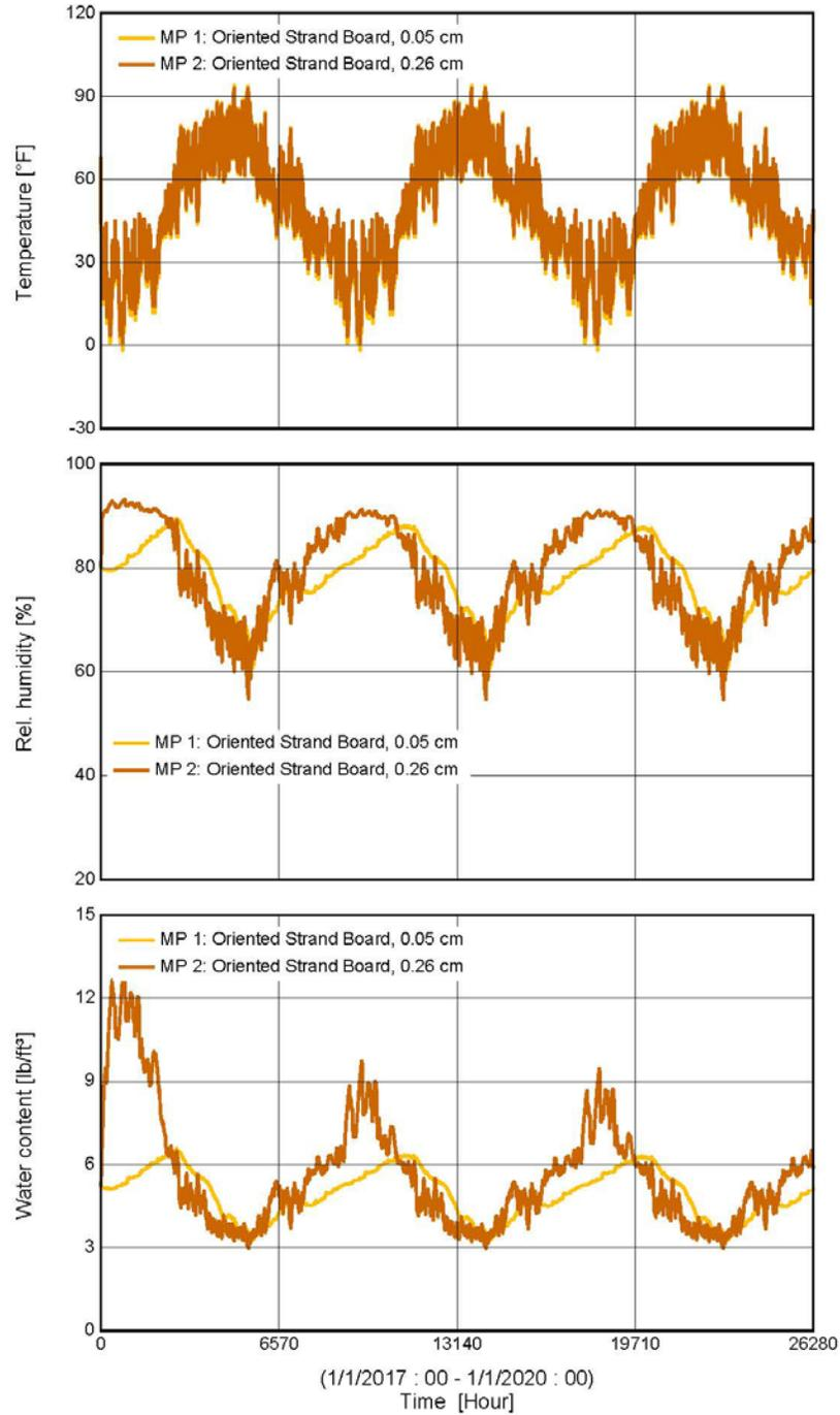
Figure E-10. 2x6 ENERGY STAR v3 wall sheathing temperature, RH, and moisture content (yellow = outer, brown = inner surface)
