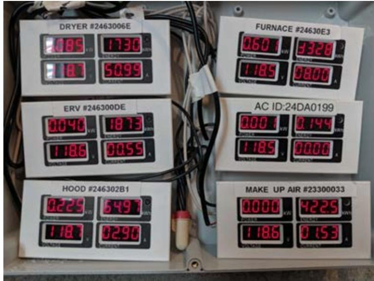
Figure 6. Electric current monitors
