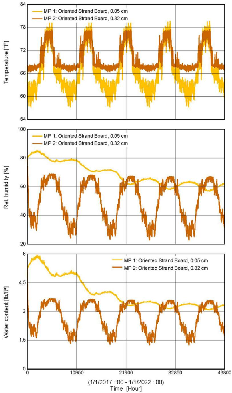
Figure E-12. SPS wall structural panel temperature, RH, and moisture content (yellow = outer, brown = inner surface)
