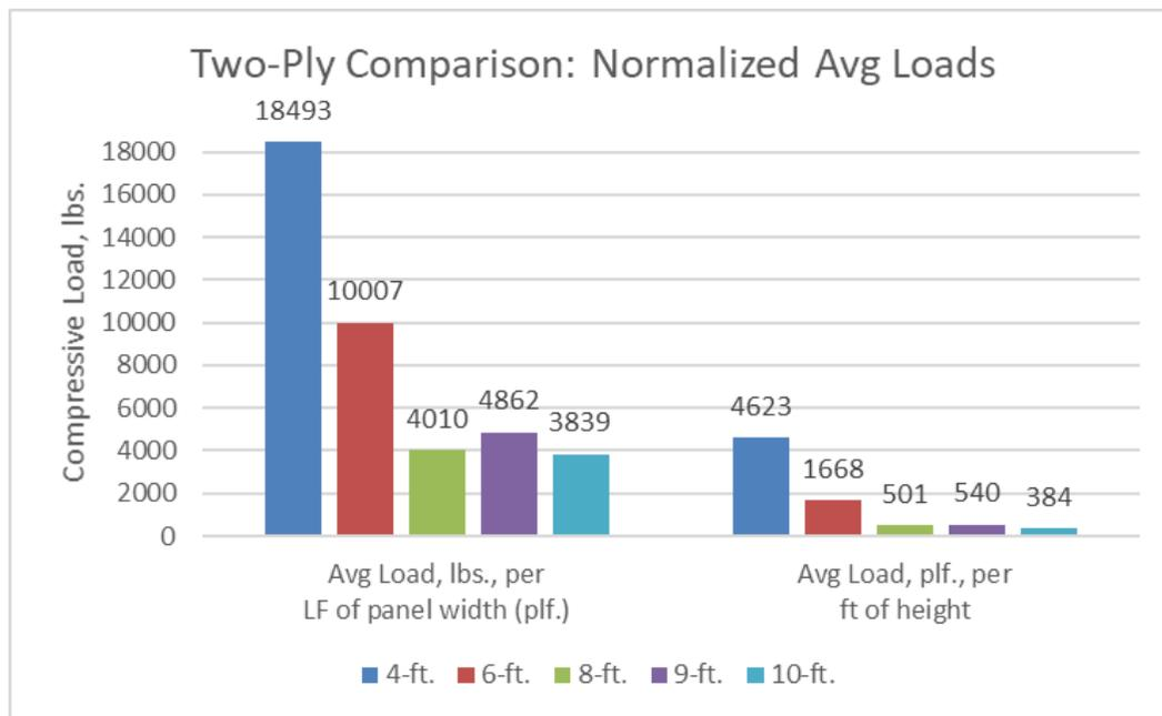
**Figure 18. Normalized average loads for 2-ply—all specimen heights**
