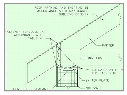
Figure 4.3 SIP Wall to Roof Connection
