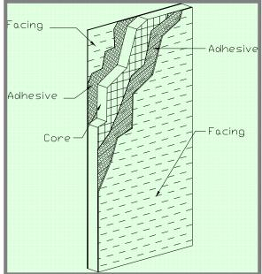
Figure 2.1 Cross Sectional View of Sip
