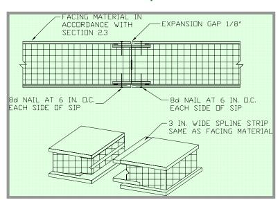
Figure 6.1 Surface Spline
