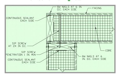
Figure 6.3 SIP Corner Framing Detail
