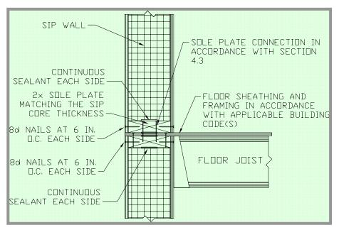
Figure 4.5 SIP Wall to Wall Balloon Frame Connection
