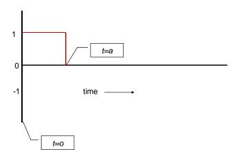
The algebraic addition of a unit step and a negative time shifted unit step creates the foundation of the signal we are looking for. Mathematically it is modeled by:
