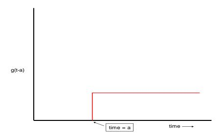
Notice that the signal we just agreed to define has an amplitude of either 0 or 1. When  $(t-a) \ge 0$  we will call this signal with an amplitude of 1 as a unit step.
