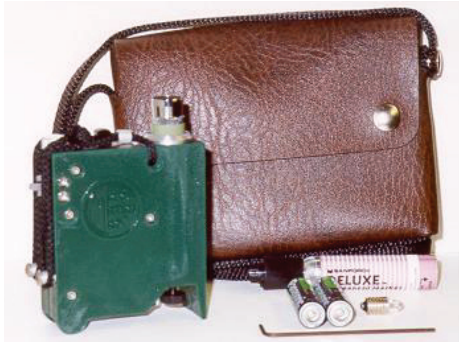
Figure 2.1.29 Tooke Gage Used to Measure Coating Dry Film Thickness
